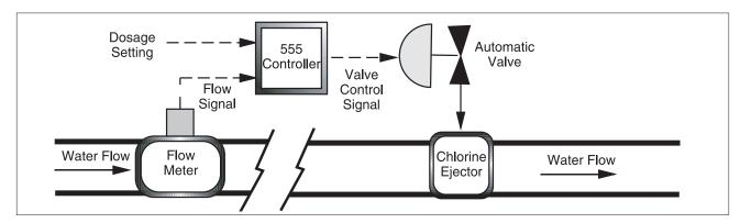
Flow paced (or flow-proportioning) control positions a chlorine or sulfur dioxide valve in direct proportion to the water flow rate. For chlorine, a user-defined "dosage-setting" from 0% to 400% (the percentage of gas flow to water flow) increases or decreases the rate of gas feed dependent on water flow rate. Similarly, a 0% to 400% dosage setting is also available for dechlorination with sulfur dioxide.
