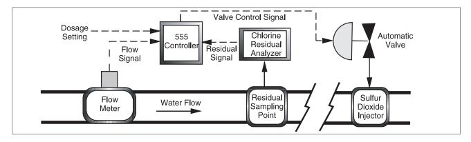
Feedforward dechlorination control positions a valve (typically sulfur dioxide) in direct proportion to the water flow rate (flow-paced on water) and residual level. With a user-defined "dosage-setting" settable from 0% to 400% (the percentage of gas flow to water flow), the 555 increases or decreases the rate
